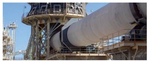
That is accomplished by skewing the roller shafts at slight angles to the rotary kiln shell and it is also known as training the kiln.
