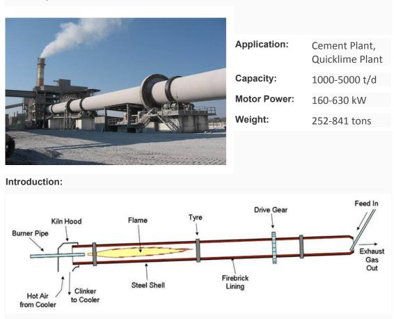
Rotary kiln is a pyroprocessing device used to raise materials to a high temperature (calcination) in a continuous process. Materials produced using rotary kiln include: Cement,
