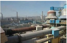
Material will be feed into kiln tail through chute in gas chamber. As kiln shell is inclined and it rotates slightly, material will move along round shell and will also move along shaft direction from kiln tail to kiln head. Material will be processed through pre-heat, decompose, calcined and will be feed into cooler. Fuel will be
