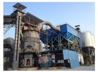
Equipment Type: GRMS46.41 Slag Vertical Roller Mill Power Consumption of System: 38 kWh/t Standard Production Capacity: 105 t/h Annual Output: 600,000 tons GGBFS Effective Diameter of Millstone: 4600 mm The feed water: max.15%H2O Number of roller: 4 Specific surface: 4200~4500cm2/g
