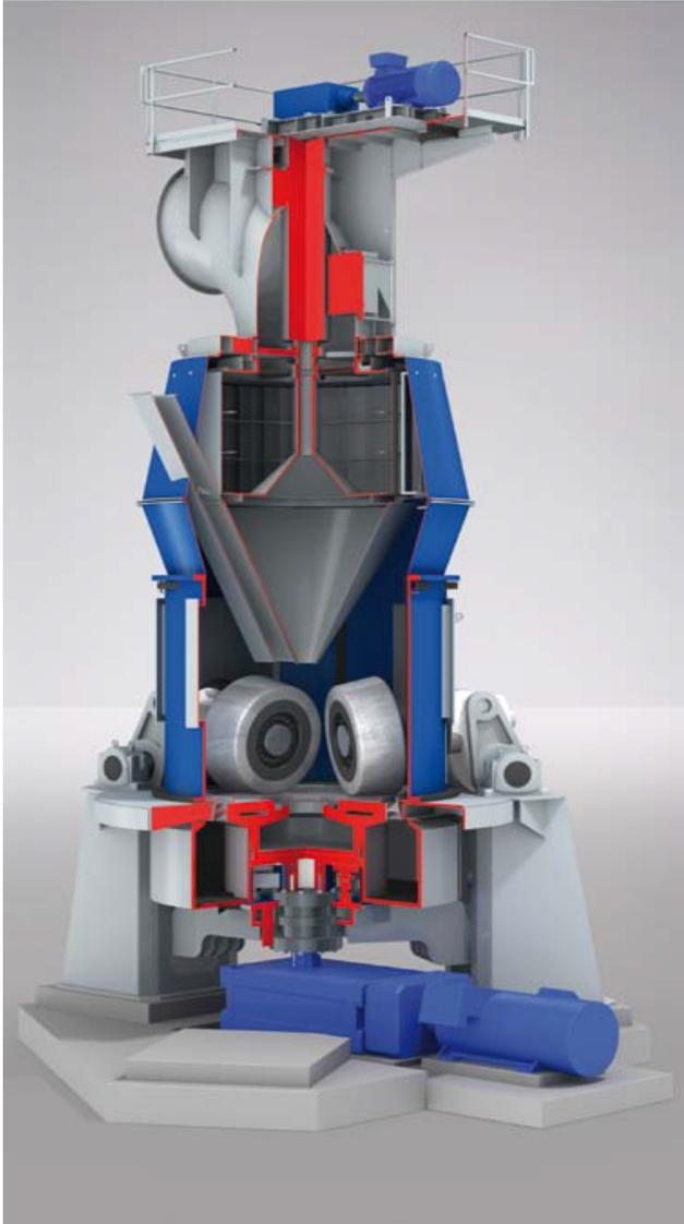
Vertical roller mill is a completely new and innovative design and a further step to more efficient grinding of soft and medium-hard products. The basic concept is based on a combination of the lower section of the mill featuring the roller and its supports, the grinding table and drive system, together with a series of highly efficient classifiers. Depending on the different product requirements the mill can be equipped with different types of separators.
