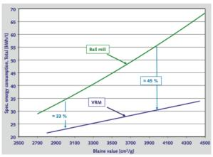
Traditionally, the closed circuit ball mill with high efficiency separator has been the most common system for cement grinding. However, as happened with raw grinding over the last 25 years, the vertical roller mill (VRM) is now successfully being used for many clinker grinding applications and is rapidly becoming the standard for new grinding installations. The first such <u>vertical roller</u> <u>mill</u> installation in the United States was
