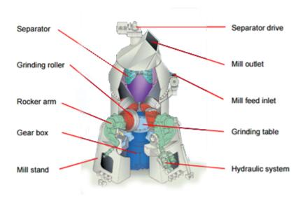
The differences between raw and cement grinding have been well documented in numerous publications and presentations over the recent past. Specifically, as compared to limestone, clinker and cement raw materials are finer and harder to grind. This, coupled with the finer and more stringent product particle size distribution requirements, entails design considerations to allow for continuous and stable operation of the grinding system.
