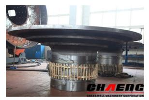
Ball mill trunnions and heads are subject to large alternating stresses during operation. Even though ball mill trunnions are designed for infinite life, there is always a risk of cracks developing due to small casting defects, wear of the inner surface of the trunnion or other damage, such
