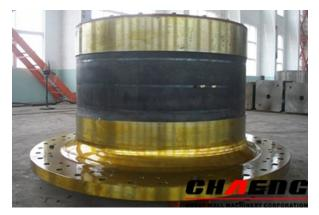
If wear or a crack is discovered in a trunnion, great wall can provide provisional on-site repair so that the mill can keep operating until a new trunnion is supplied. Any weld repair of a trunnion must be considered as a temporary solution since new cracks will most likely develop and the repair can result in trunnion deformations, which can cause bearing problems and eventually lead to bearing failure. Therefore, it is strongly recommended to order and install a new
