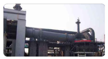
The <u>rotary kiln</u> is a refractory lined cylinder rotating about its axis. The rotary kiln slopes slightly downward from feed to discharge end. The slope and rotation of the kiln move the material through it. Rotary Kiln speed is variable to vary pellet retention time. The rotary kiln is a single chamber with an open feed end connected by housing to the grates preheat furnace.
